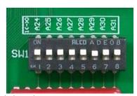
Example: DIP-SW Address above is : 0x00000000, Extended Mode
